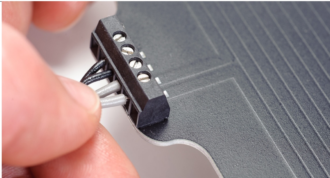
image 76: Connecting the Heated bed Cable.
